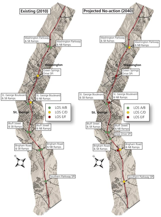
Figure 1-3 Existing (2010) and Projected No-action (2040) PM Peak Intersection LOS
