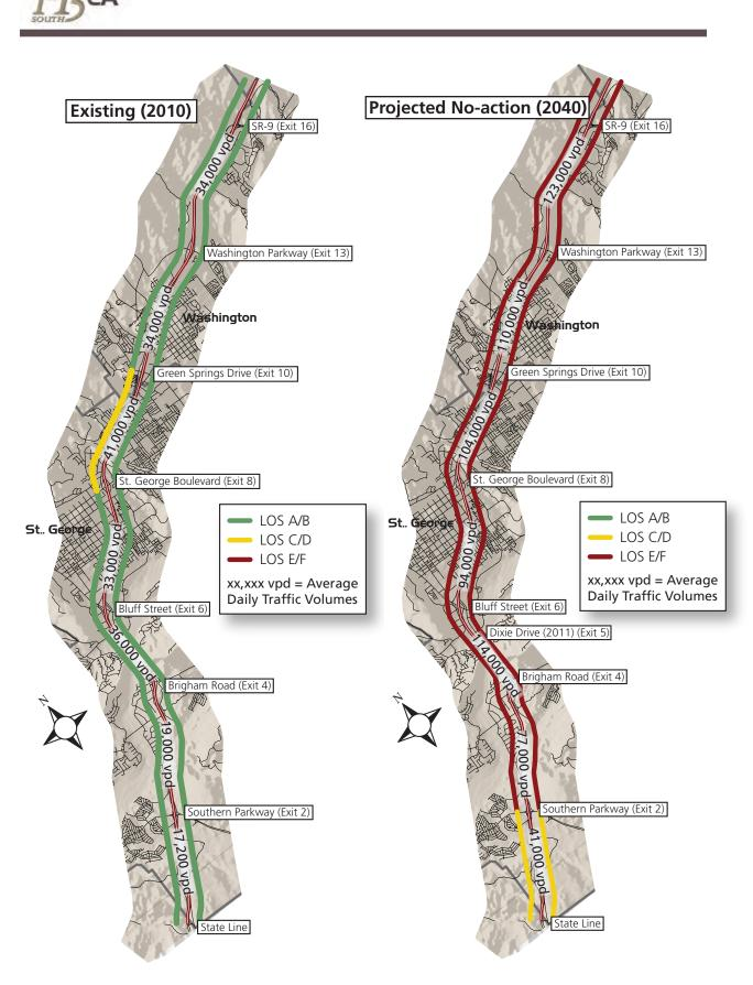
Figure 1-2 Existing (2010) and Projected No-action (2040) Traffic Volumes and LOS
